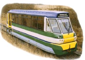
Now, frankly, it was a bumpy ride in parts because of the freight-only track and because the four wheels, close together are not on a sprung bogie, but the next development, specially planned to be trialled on the Wensleydale line will be a bit like a 'bendy-bus' with sprung bogies.
